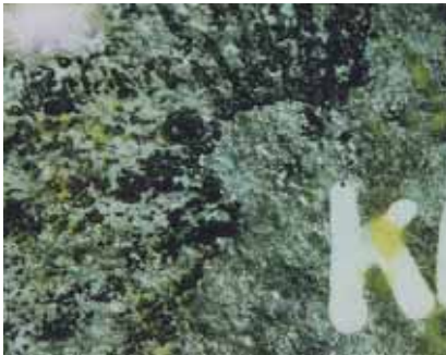
3 Microphotograph (6 x 9 mm) of black spots on the reverse and residues of the yellow plastiline. The area around the inventory letters has been protected by a lacquer.
